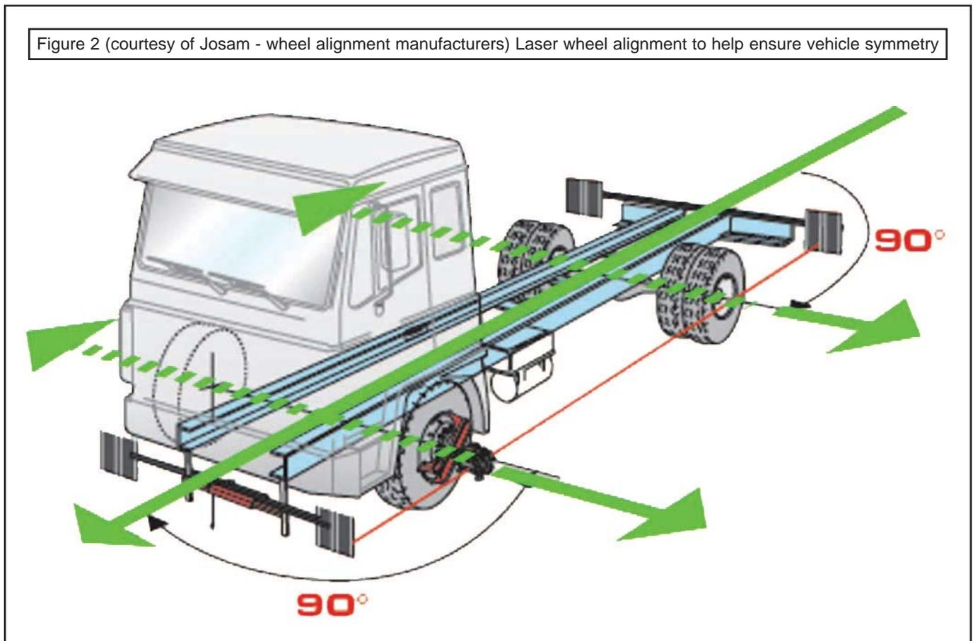
The process of laser wheel alignment involves fitting the vehicle at the front and rear with bars with measuring gauges attached. Devices are then fitted to each wheel, complete with laser lights. These laser lights on each wheel are lined up with the gauges on the front and rear bars, to measure the amount of 'toe in' and 'toe out' of each wheel. Having taken these measurements, simple adjustments can be made and wheel realignment achieved. Figure 2 illustrates the procedure.
