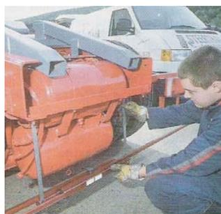
Bars with measuring gauges fitted front to rear
