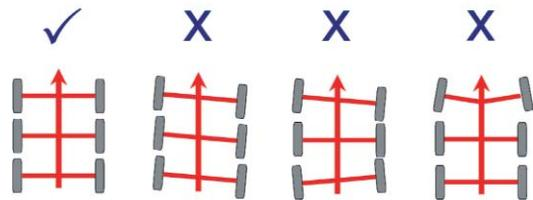
Figure 1: Correct wheel alignment
